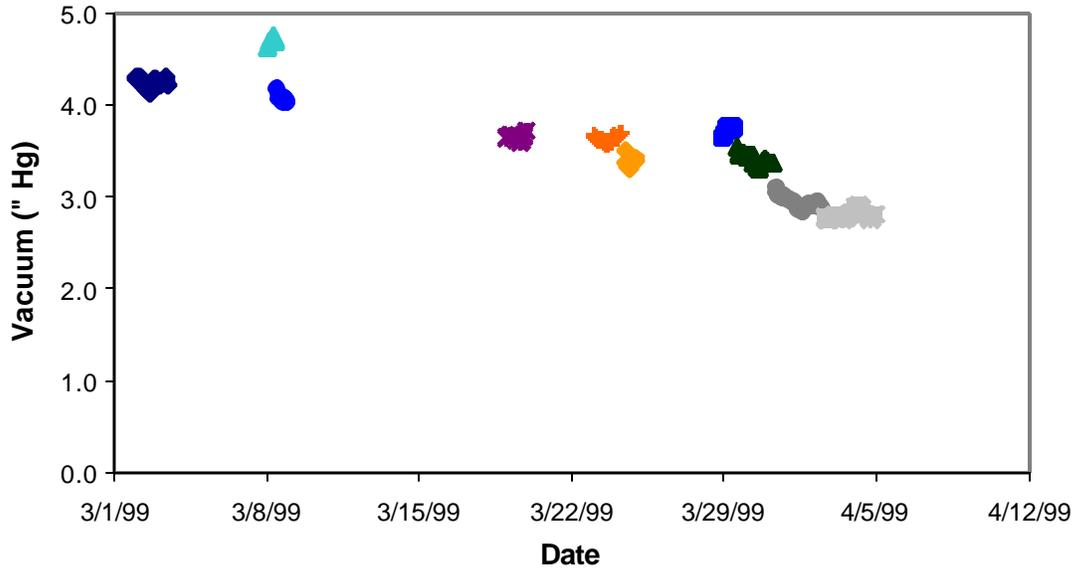
**Figure 14. Vacuum vs. Days After Chemical Cleaning
