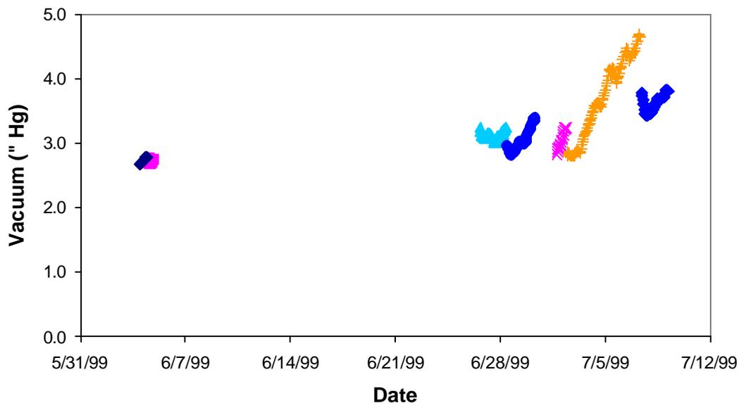
Figure 16 shows the vacuum as a function of the elapsed time from a chemical cleaning. The vacuum ranged from 2.7 to 4.7 "Hg and increased at a rate of approximately 0.19 "Hg per day after chemical cleaning.
