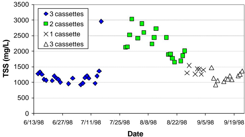
TSS removal appeared to be unaffected by the high concentration of solids in the reactor. The permeate TSS ranged from <0.4 mg/L (the detection limit) to 8 mg/L over the first two weeks of testing. Afterwards, the value remained consistently below 1.0 mg/L. As seen in Figure 4, the microfiltration unit removed 99.9 percent of the TSS.
