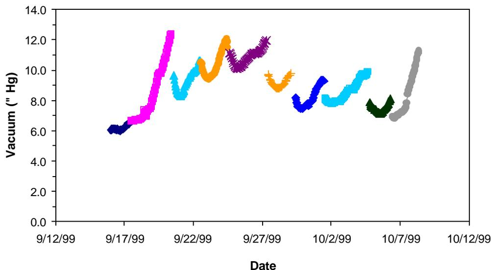
Figure 20 shows the vacuum as a function of the elapsed time from a chemical cleaning. The vacuum for this test period ranged from approximately 6 to 12 "Hg and increased an average of approximately 1.05 "Hg per day. The data show substantial scatter, even immediately after a chemical cleaning. As in the low concentration, high flux test, there may be some small cyclic variation visible in the data, but it is not pronounced and may reflect normal data scatter.
