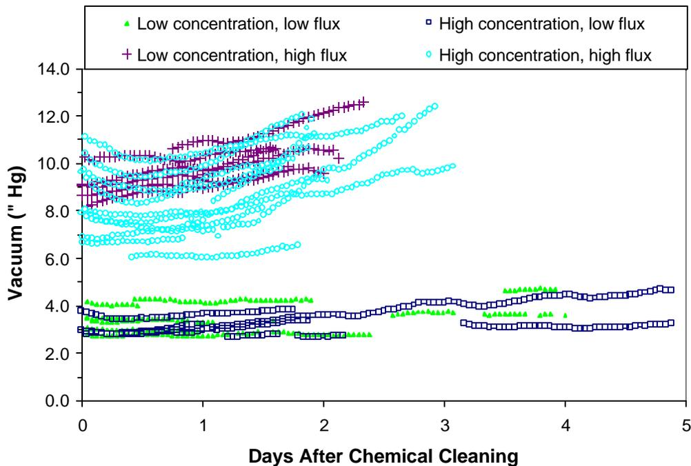
The operating vacuum increased at higher flux conditions. The difference in vacuum between the two flux conditions averaged 4 to 6 "Hg even immediately after a chemical cleaning. One would expect that forcing more flow through the pores in each time interval would require a greater driving force, so this result was not surprising.
