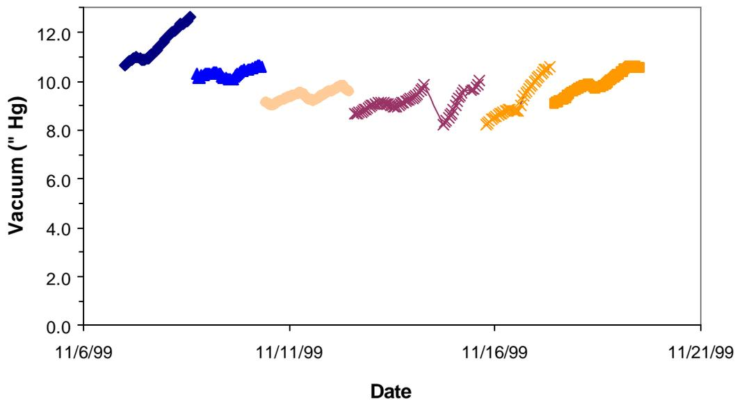
**Figure 18. Vacuum vs. Days After Chemical Cleaning
