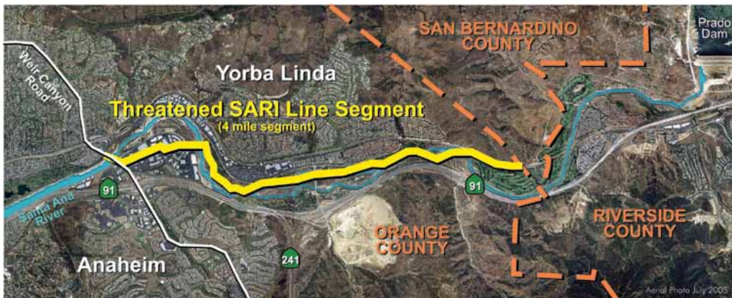
A four-mile segment of the Santa Ana River Interceptor pipeline will be rerouted out of the riverbed to protect the sewer system from erosion.
