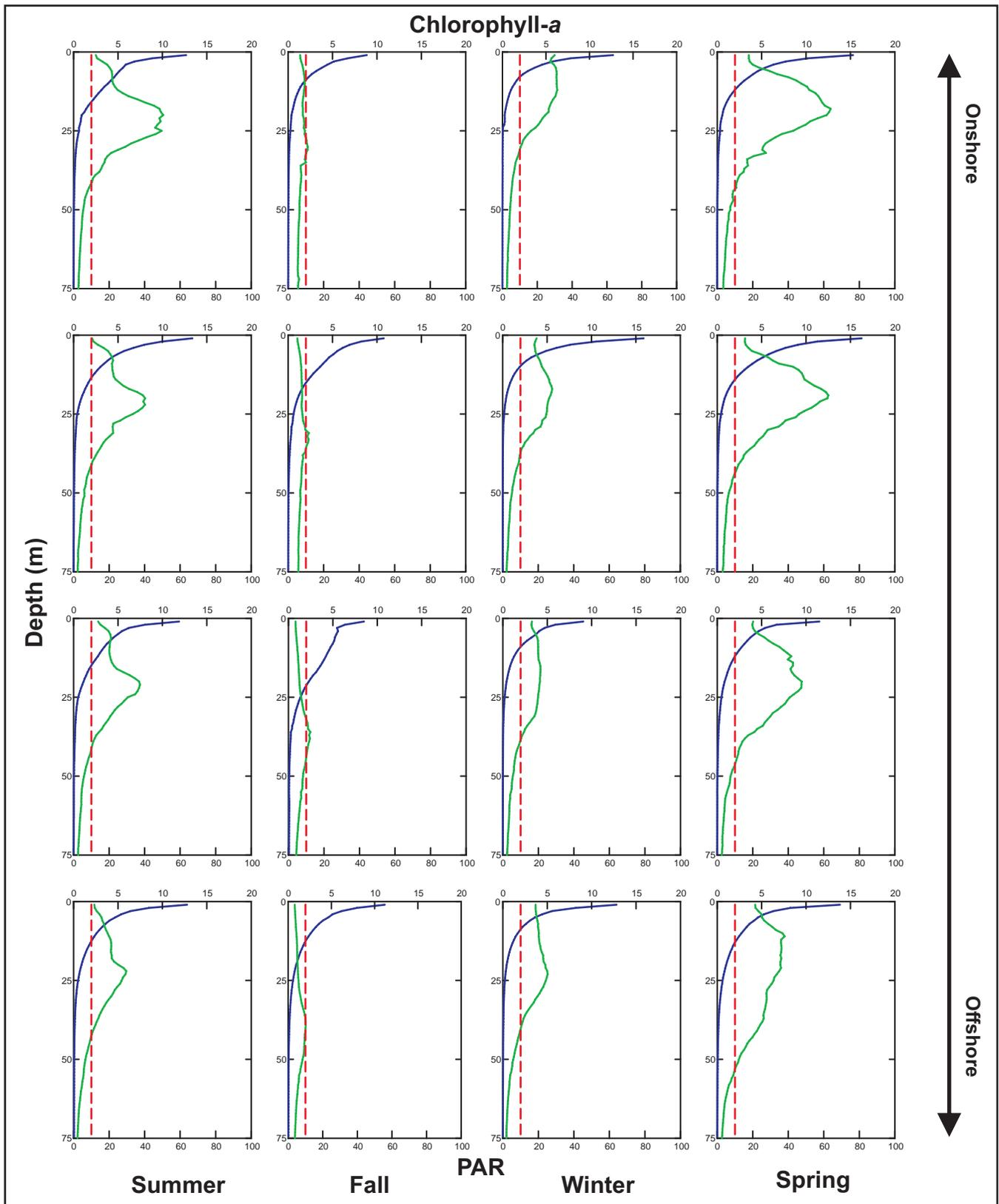
**Figure 3-19. Quarterly average chlorophyll-a fluorescence ( $\mu\text{g/L}$ ; green line) and photosynthetically active radiation (PAR;  $\mu\text{E}/(\text{cm}^2\text{-sec})$ ; blue line) with depth for summer (August 2009), fall (November 2009), winter (February 2010), and spring (May 2010). Red dashed line represents the 10% light penetration level.**
