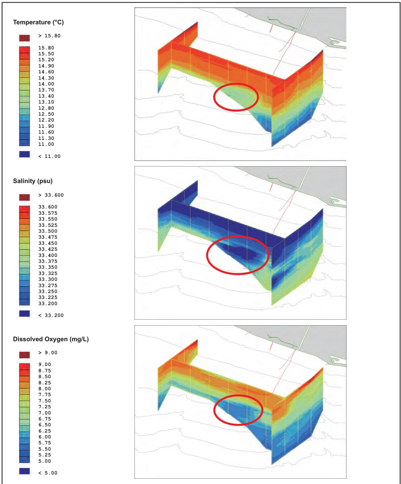
**Figure 3-12. Examples of plume-related changes (circled in red) in temperature (°C), salinity (psu), and dissolved oxygen (mg/L) near the outfall on February 17, 2010.**
