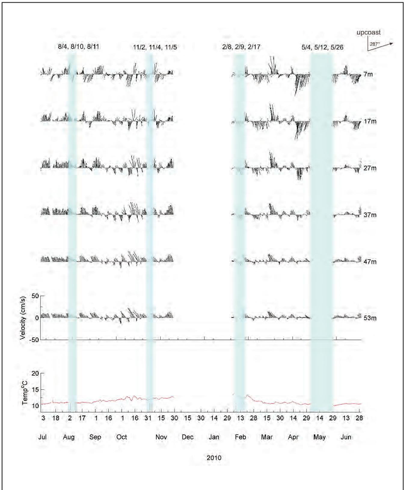
Figure 3-8. Bottom temperature (°C) and current speed (cm/s) and direction by depth for mooring M21, July 2009–June 2010. Blue lines denote water quality sampling events.
